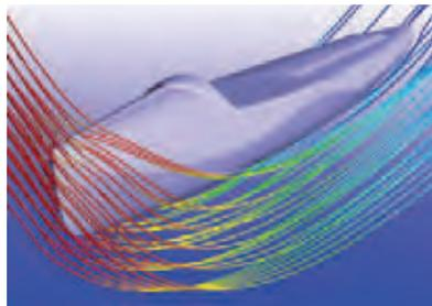
Using computer simulation, Intelligent Fluid Solutions designed a more stable and better-draining surfski for Red7 without compromising speed. Top racers confirmed improved times, and sales of the product increased.
