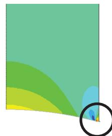
**A 2-D axisymmetric model shows contours of equivalent stress on punch head during contact with tablet. The red area at lower edge corresponds well with experimental results indicating the location where the punch head is most likely to break down.**
