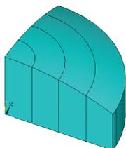
**Structural model of representative tablet shape with a constant Young's modulus (top); tablet that has been divided into four sections (bottom), in which the variable Young's modulus is transcribed for each section by computed reaction force on the punch head. Both models employ symmetry to speed up calculations.**
