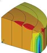
**Contour plots showing maximum principal stress on tablet when load is imposed at lower right edge (blue and green colors): model with one section (top), two sections (center) and four sections (bottom)**
