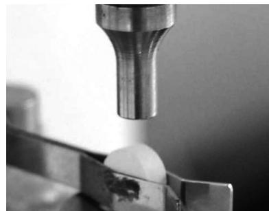
Pharmaceutical and food industries define tablet hardness as the load from one direction that is required to break a tablet.
