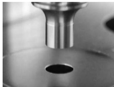
The process of tablet formation begins when powdered raw material is fed into the punch hole from below. The punch presses down into the hole and compacts powder into the cavity, under pressure, to harden it into a tablet. After depressurization, the punch head lifts up, and the device ejects the tablet.
