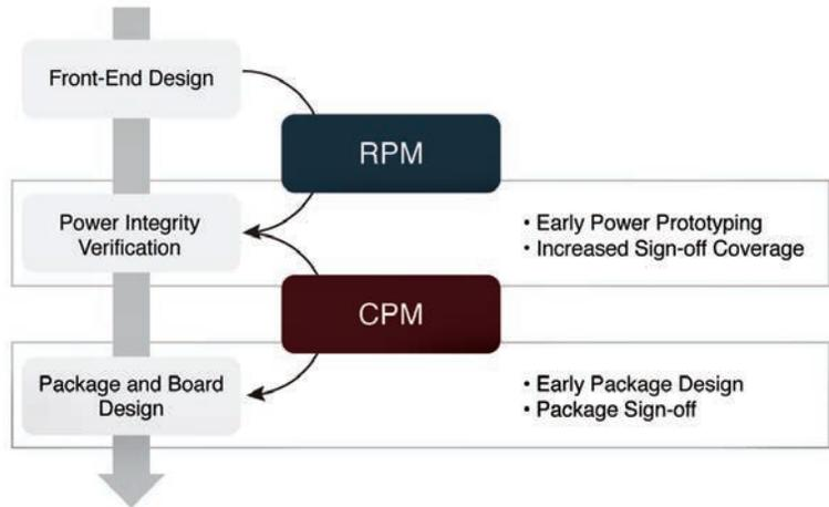
**RTL-to-physical power integrity flow using RPM and CPM**
