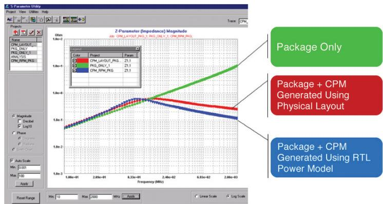
**Package resonance frequency analysis: tight correlation between RPM vs. layout**
