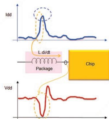
Lowering power adds additional PDN integrity challenges. A surge in current causes voltage-induced timing failure.
