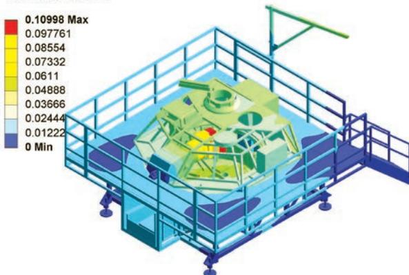
**Static structural analysis results on initial design showed excessive deformation in several areas.**
