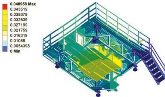
**Static structural analysis results of new reinforced design showed a substantial reduction in deformation.**
