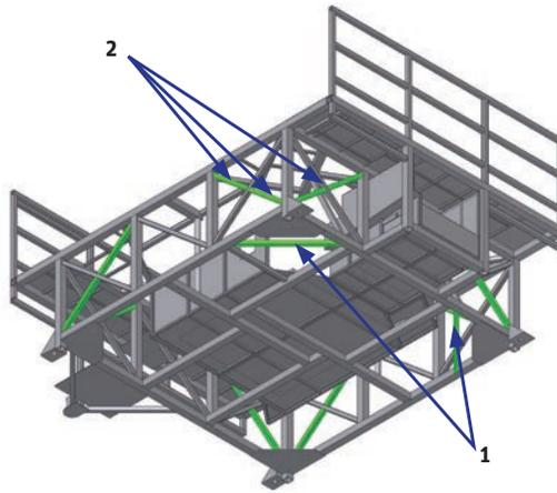
**Kratos added horizontal steel structural tubes on the bottom-frame front corners (1) as well as upper- and lower-lateral steel cross beams on each vertical post corner (2).**
