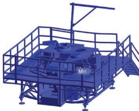
**Minimum safety factor for noncritical components in the reinforced design was 2.312, above the 2.0 design requirement.**
