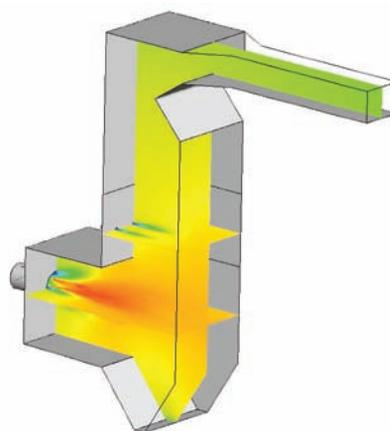
Pourkashanian and his team used engineering simulation software to predict oxy-coal combustion in an industrial combustion test facility with recycled flue gas to address the major technical challenges of using this system for power generation with carbon capture and sequestration.
