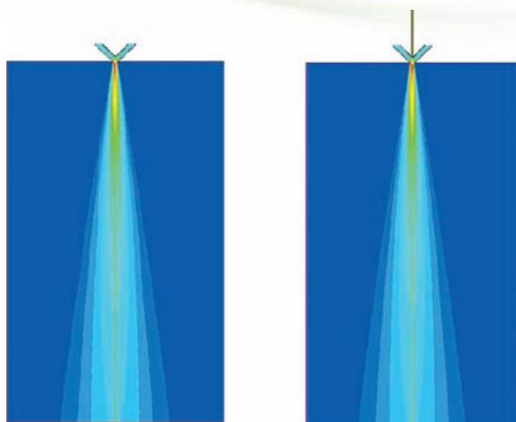
Pourdeyhimi's research group uses ANSYS Fluent software to model air flow fields during melt-blowing production processes for nonwoven fibers. During melt blowing, molten polymer streams are injected into high-velocity gas jets, and polymer fibers are attenuated by the resulting drag force.
