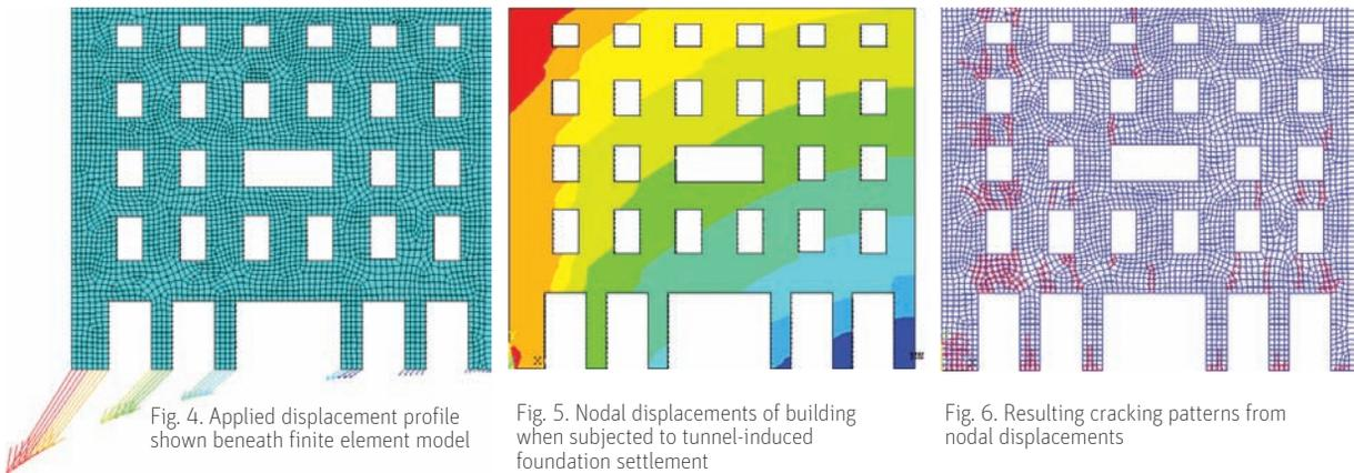
Fig. 4. Applied displacement profile shown beneath finite element model
