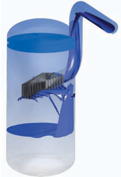
Analysis of a vertical production separator with a vane-type inlet device shows that the inlet pipe keeps much of the liquid on one side of the vessel — leading to non-optimal separation.
