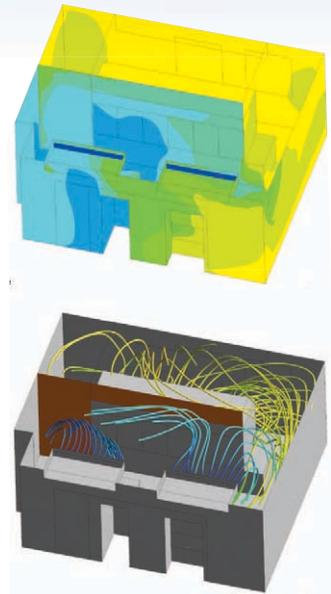
Addition of a simple thermal partition significantly improved temperature uniformity and airflow.
