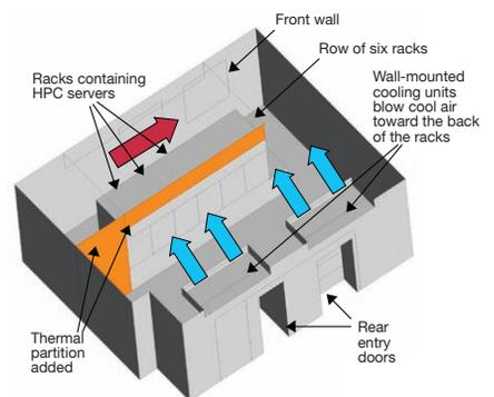
Constructing thermal partitions (highlighted) at the top and one side of the racks was a quick and inexpensive way to modify airflow for correcting the overheating problem.
