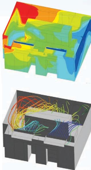
Contour plot (top) shows hot spots resulting from hot airflow traveling over and around the rack units directly back into the rack inlet. This hot airflow pushes cooling air partially away from the HPC racks to further increase air temperature drawn into the racks (bottom).
