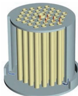
Configuration of a 36-tube anode-supported SOFC stack
