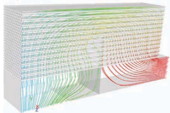
Flow speed and temperatures through the tubes in the air-air cooling system
