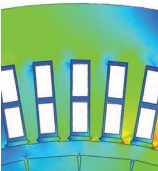
Magnetic flux density level in the stator (left) identifies areas of high losses. The generated voltage (upper right) and fast Fourier transform (FFT) (lower right) results for a no-load condition are also shown.
