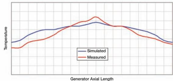
The difference between the simulated and measured air flow rates across the length of the generator was a maximum of 1.32 percent. The maximum difference in calculated versus measured temperatures was only +/- 3 degrees C for the stator and +/- 3 degrees C for the rotor magnets. Software from ANSYS provided very good accuracy, which is essential for these applications and for Indar engineers to trust the new design variations.
