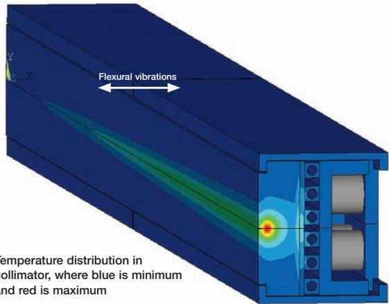
finite element analysis software provides multiphysics capabilities that integrate thermal and mechanical analysis. In this application, integration increases accuracy and reduces the amount of time required to prepare the model. ANSYS Mechanical also offers comprehensive element technology, an extensive library of material models, auto contact detection for assemblies and powerful solver capabilities.
