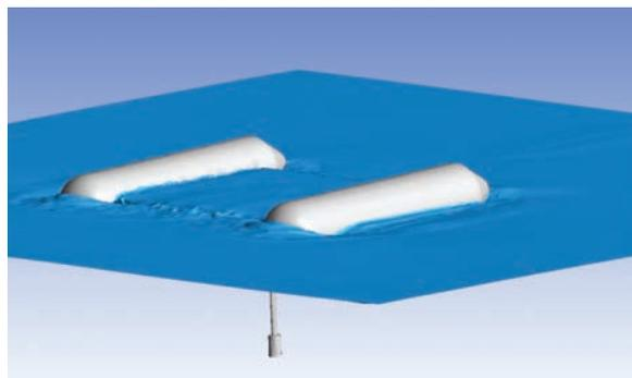
Sensor float bow nosing down due to flow on sensor below float, deck awash
