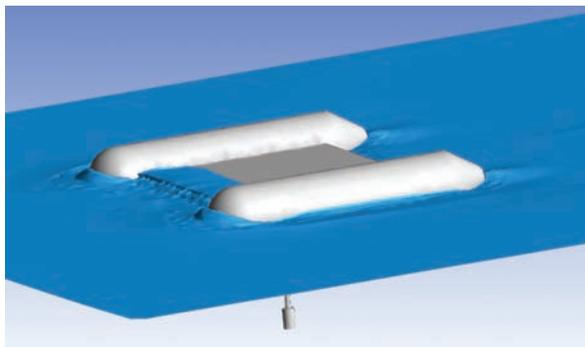
Sensor float fluid–structure interaction (FSI) transient response to current flow
