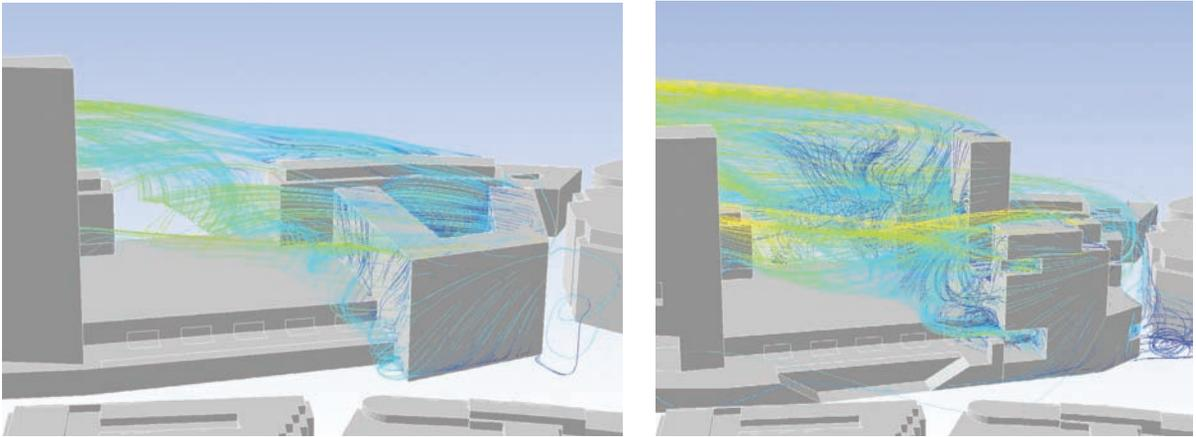
Pathlines showing wind trajectory colored by velocity magnitude for original (left) and new (right) designs provided increased understanding of wind behavior near buildings to determine areas of concern.
