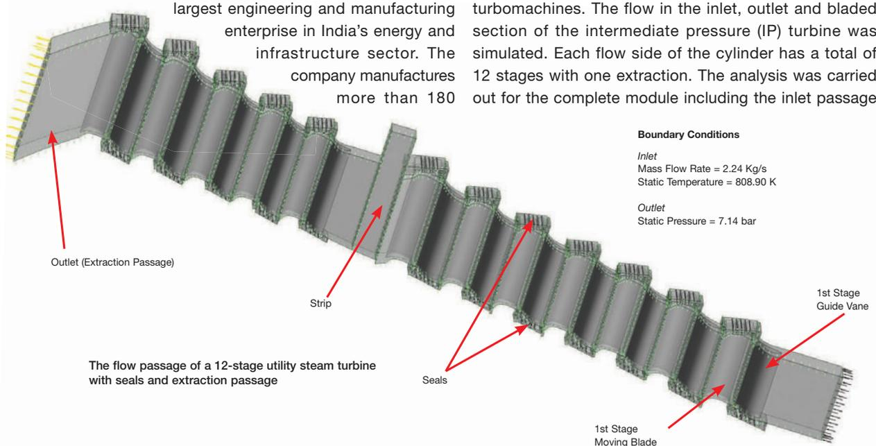
section, bladed path with seals, steam extraction and outlet passage section of the turbine. The model consisted of a single blade passage for each blade row including the seal and interface regions for a total of 24 blade rows and 50 components. The engineering team generated blade row meshes using the ANSYS TurboGrid tool and employed ANSYS ICEM CFD software to generate the mesh for the seals, inlet and outlet passage sections.
