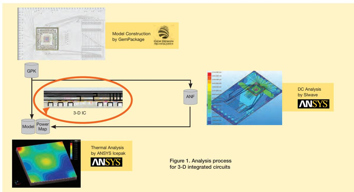
Figure 1. Analysis process for 3-D integrated circuits
