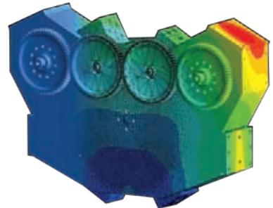
Stress distribution of the CHB engine housing overlaid on the geometry and mesh of the ANSYS Mechanical model
