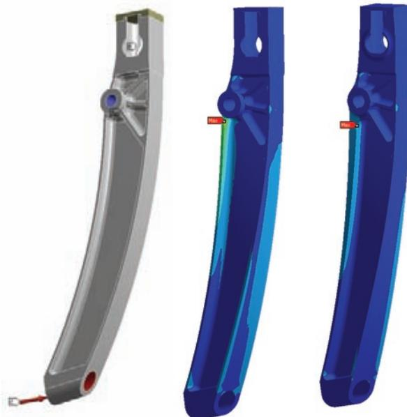
Pedal failure corresponding to the ANSYS stress plot, showing how the model was restrained and loaded: loads and constraints (left), original design (middle) and optimized design (right)
