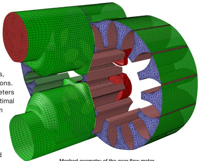
Meshed geometry of the gear flow meter
