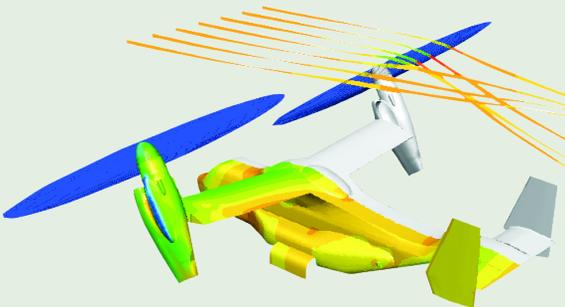
The dynamic mesh model is one of the moving and deforming mesh capabilities available in ANSYS tools for fluid flow simulation. The moving mesh technology in ANSYS FLUENT software can be used to model the changing tilt of the rotorcraft's wings while changing flight modes, illustrated with this Osprey aircraft.
