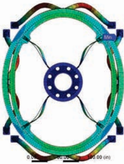
Telescope and camera assembly at mode 6 natural frequency of 14.006 Hz
