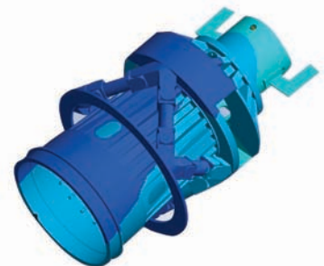
Barrel and imager Z direction displacement under vacuum load, thermal load and gravity load at 20-degree C ambient temperature
