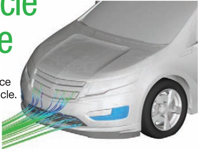
CFD was used extensively to develop the front-end cooling airflow characteristics of the Volt.
