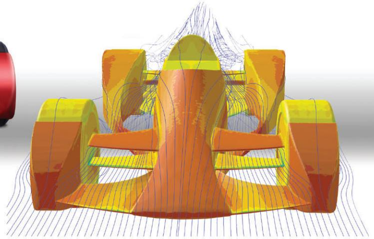
Fluid dynamics software from ANSYS was used to determine the aerodynamics of a concept F1 racecar.
