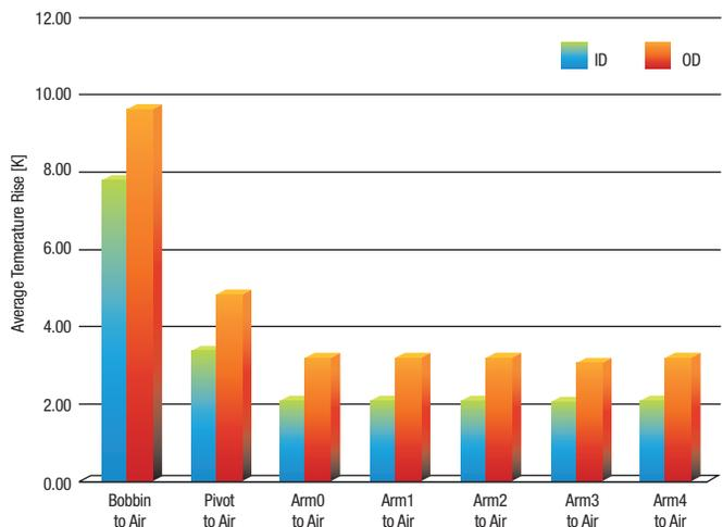
Temperature rise in different locations in the head stack assembly of a hard disk drive with the actuator arm in different positions (ID – inner diameter, OD – outer diameter)
