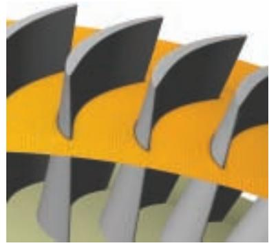
New developments in the ANSYS TurboGrid software are used to create high-quality meshes for bladed components with minimal user input. Geometry courtesy PCA Engineers.
