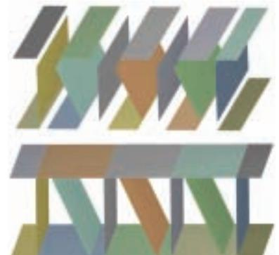
Improved surface extension: Users can select and extend multiple groups of surfaces in a single step, a procedure that greatly simplifies the process of closing gaps between parts after mid-surface extraction. The images show a sample model before and after surface extension.
