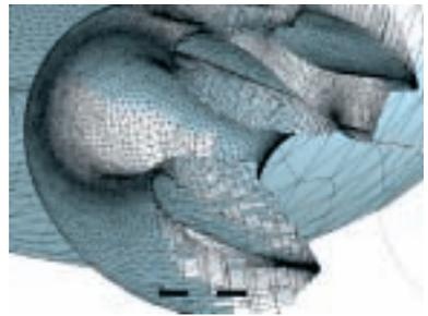
Patch conformal tet method with advanced size functions: With minimal input, ANSYS size function-based triangulation and inflation technology can handle advanced CFD meshing challenges, such as this benchmark aircraft model.
