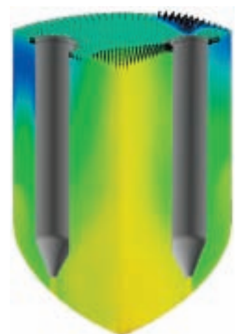
At the end of the drive phase, higher concentrations are predicted at the top boundary of the fluid domain while concentrations were reduced at the bottom as the solids were pushed away from the jet nozzle exits.
