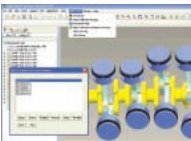
Named selection manager: This new feature allows a user to create and save named selections within CAD systems and then to use them within ANSYS applications. This example uses the named selection manager within Pro/ENGINEER.
