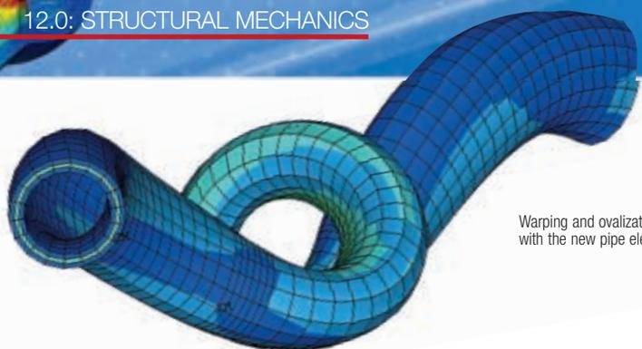
Warping and ovalization of pipe structures with the new pipe elements
