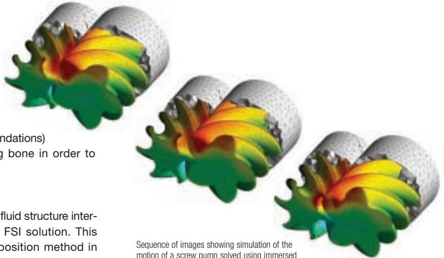
Sequence of images showing simulation of the motion of a screw pump solved using immersed solid fluid structure interaction
