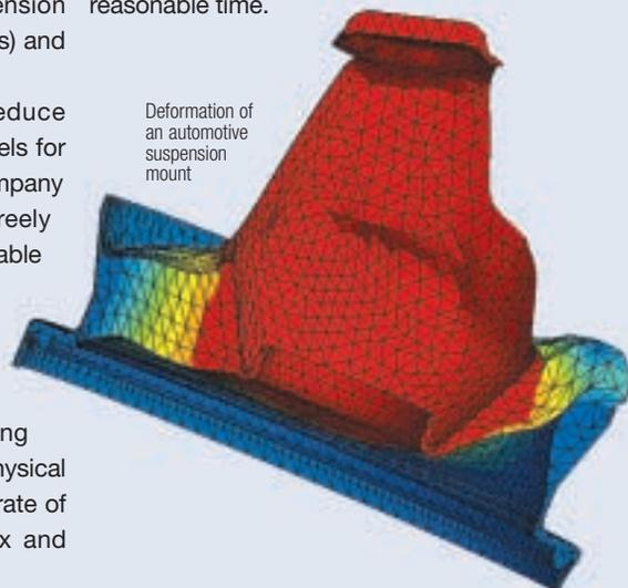
Deformation of an automotive suspension mount
