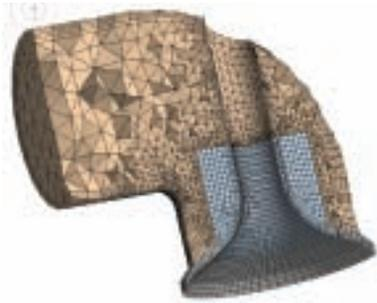
Hybrid mesh: Using a combination of sweep and tetrahedral mesh methods, a user can quickly control the mesh in regions of interest to improve the accuracy of the solution without the need for a pure hex mesh (and the time required to generate it).
