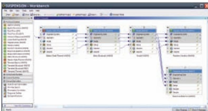
More-complex analyses involving multiple physics can be built up by connecting systems. Data dependencies are indicated clearly as connections. State icons at the right of each cell indicate whether cells are up to date, require user input or need to be updated — for example, whether they are just meshed or fully solved.
