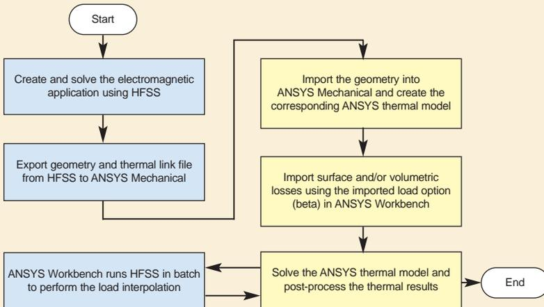
Case study procedure of one-way coupling between Ansoft (blue) and ANSYS (yellow) software
