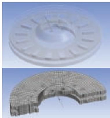
MultiZone mesh method: Using the new MultiZone mesh method, a user can mesh complicated models with a pure hex mesh without the need for geometry decomposition. This brake rotor example can be meshed with a pure hex mesh in a single operation.
