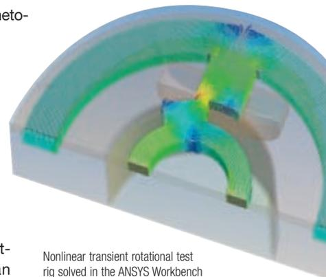
Nonlinear transient rotational test rig solved in the ANSYS Workbench environment using SOLID236, SOLID237 and the new stranded conductor option (TEAM24 benchmark)
