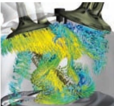
Internal combustion engine simulation is one of the focus applications for ANSYS 12.0. This snapshot from a transient simulation of the complete engine cycle shows the flow just after the intake valves open and the direct injection of fuel. New flow feature extraction options in CFD-Post are used to highlight vortex structures with velocity vectors. Image courtesy BMW Group.
