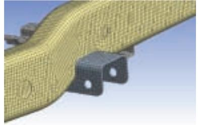
Thin solid sweep method: Using the thin solid sweep mesh method, complicated sheet metal parts can be easily hex meshed without the need for midsurfacing or welding. The mesh can be generated to conform to the shared interface to increase the accuracy and speed of the solution.
