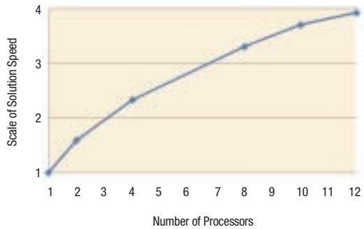
Solution scaling of a thermoelectric cooler model with 500,000 degrees of freedom enables a speedup of four times for 12 processors.
