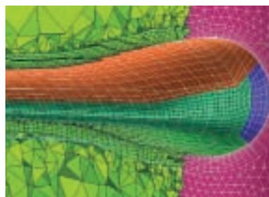
ANSYS ICEM CFD: MultiZone meshing that combines the strength of various meshing tools, automatically generated this hybrid grid for a tidal turbine.
