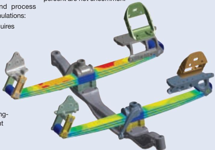
Multibody dynamics capabilities were used to simulate this leaf spring suspension.
