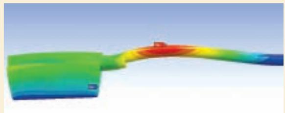
Deformation of the high-power electronic connector can be predicted by combining Ansoft HFSS and ANSYS Mechanical software.
