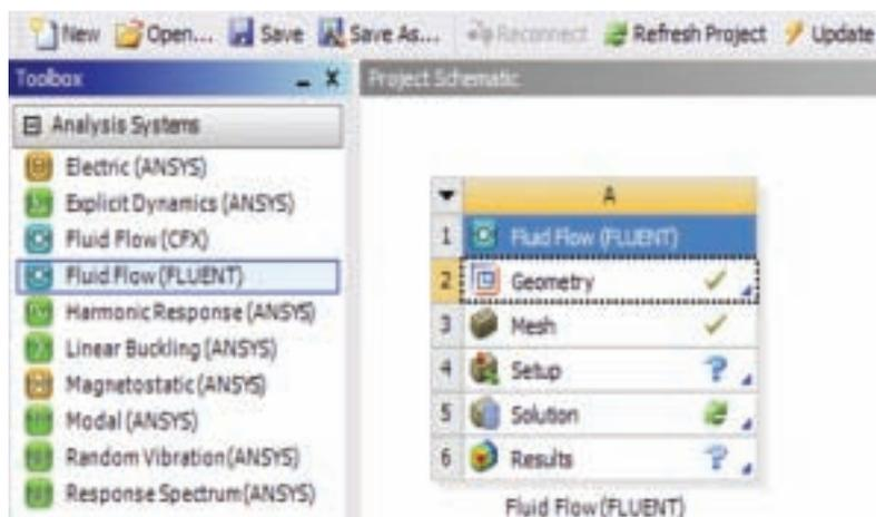
The toolbox, at left, contains systems that form a project's building blocks. In this single-physics example, the user drags the system (from left) into the project schematic (at right), then sets up and solves the system, working from the top down through the cells in the system. As shown, the Fluid Flow system (at right) is complete through mesh generation, as shown by green check marks.
