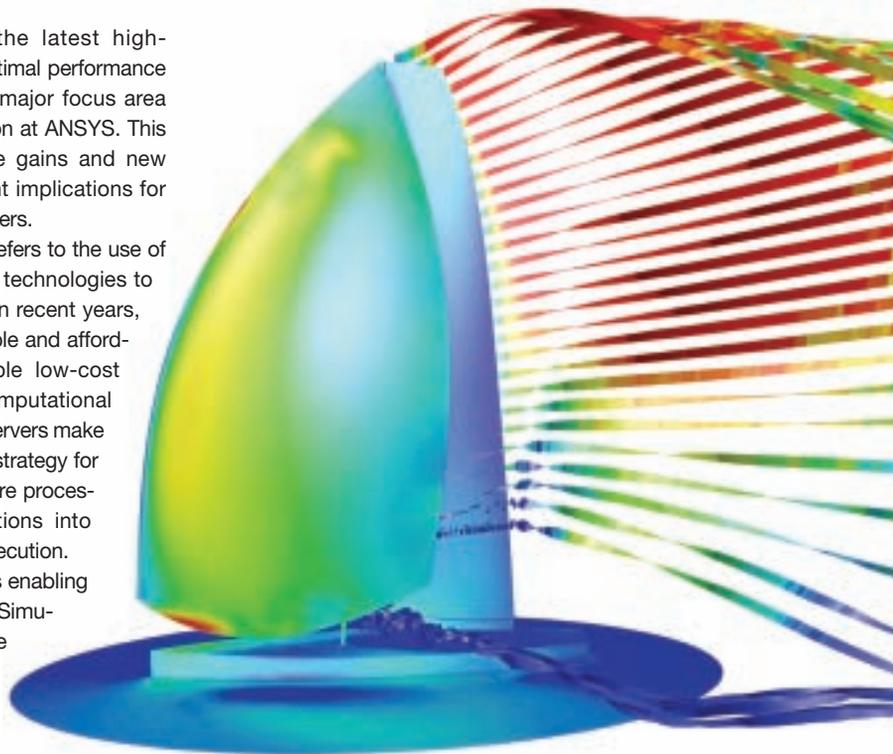
Figure 1. Simulations as large as 1 billion cells are now supported at release 12.0. This 1 billion-scale racing yacht simulation was conducted on a cluster of 208 HP ProLiant™ server blades. (For more information, visit [www.ansys.com/one-billion](http://www.ansys.com/one-billion).)
