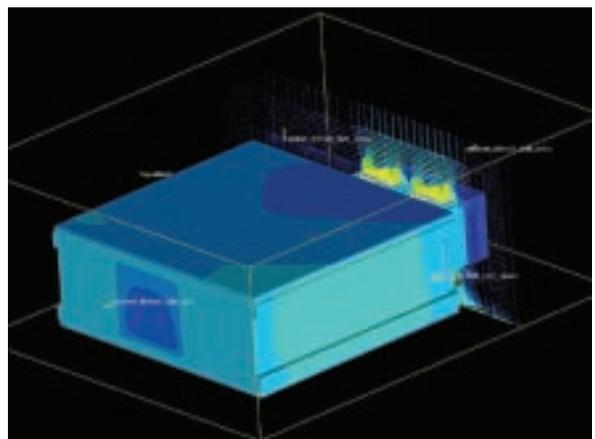
ANSYS Icepak model shows the speed of the air from the fans along with temperature contours on the chassis. Blue indicates cooler temperature.
