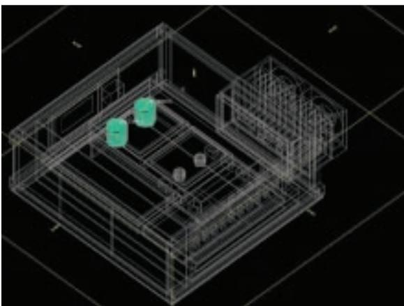
New design with aircoil filters shows that temperatures are reduced to acceptable levels. (The filter temperatures in degrees C have gone from the 200s to the 90s.)
