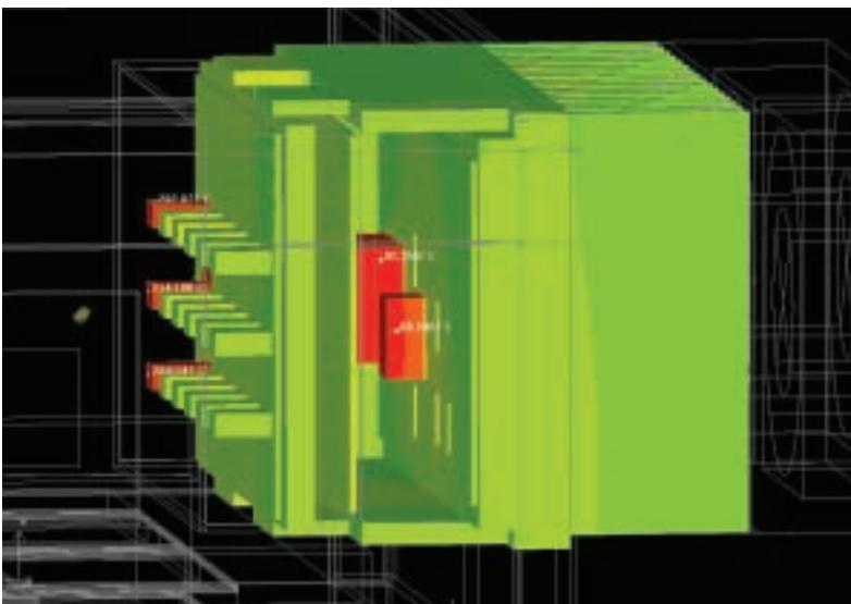
Original radio design with ferrite core filters shows hot spots.
