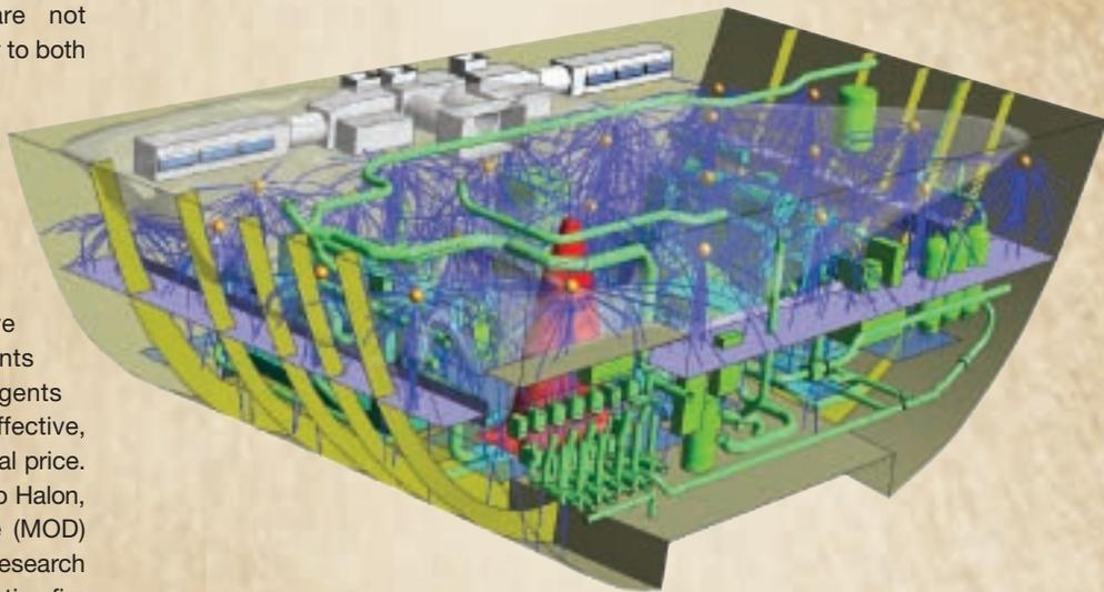
Temperature isosurfaces and droplet trajectories before fire extinction is completed in a ship's machinery space
