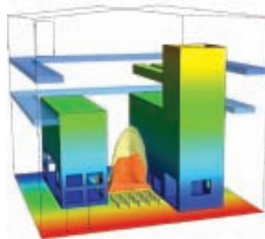
Simulation model of the rig geometry and temperature isosurfaces before spray inception
