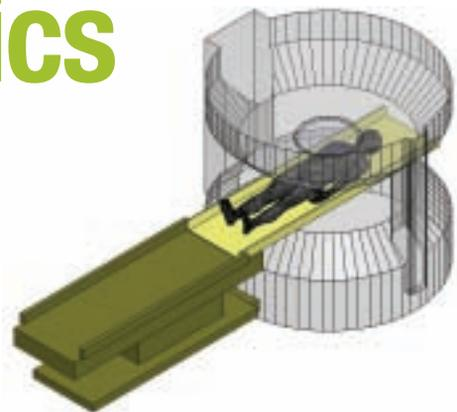
Model of the open MRI system, which combines an MRI model generated by Philips Healthcare with the ANSYS human body model
