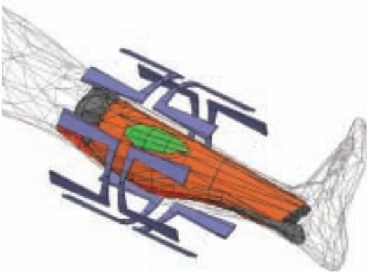
Model of a hyperthermia applicator and leg with tumor; in the image, some applicator and water cooling system components have been removed for clarity. The green object is the tumor. Applicator design and tumor geometry provided by Duke University.
