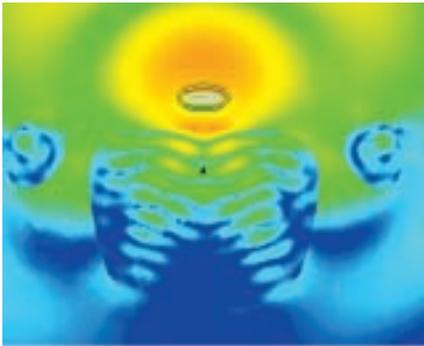
The electric field (magnitude) that results when using a receiver implanted in epidural space in conjunction with a wireless transmitter placed behind the back; the image shows a horizontal cross section of the torso and arms of a person, standing, using a wireless implant.
