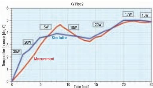
Comparison of simulated and measured temperatures in the tumor for a hyperthermia treatment case. Measured results provided by Duke University.
