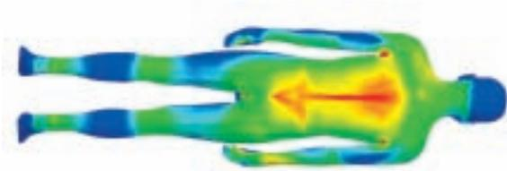
Sample of specific absorption rate that results on the body when using the open MRI system, as simulated using the HFSS electromagnetic field simulation tool
