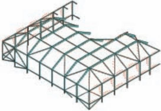
APDL is used to automatically create, load and solve a full-frame model of a screen enclosure from parameters entered by the user describing the structure.
