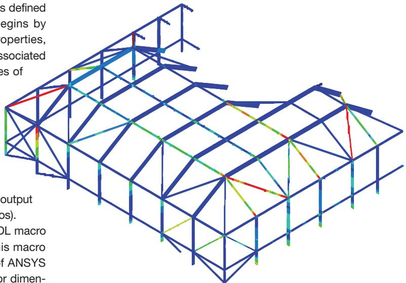
Color contour plots of interaction ratios show locations' potential wind-force failure in red.
