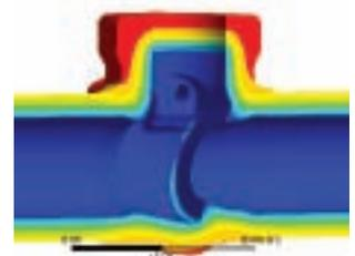
Temperature distribution in the valve at 532 seconds into a transient analysis of the valve behavior during a shutdown event
