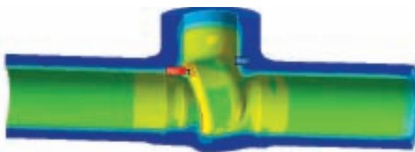
Stress distribution in the valve at 532 seconds into a transient analysis of the valve behavior during a shutdown event
