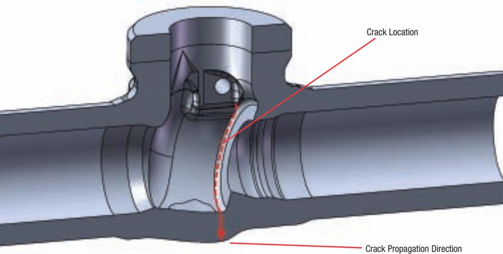
The valve model showing the location of the crack on the inner surface of the valve and the direction of propagation of the crack through the wall
