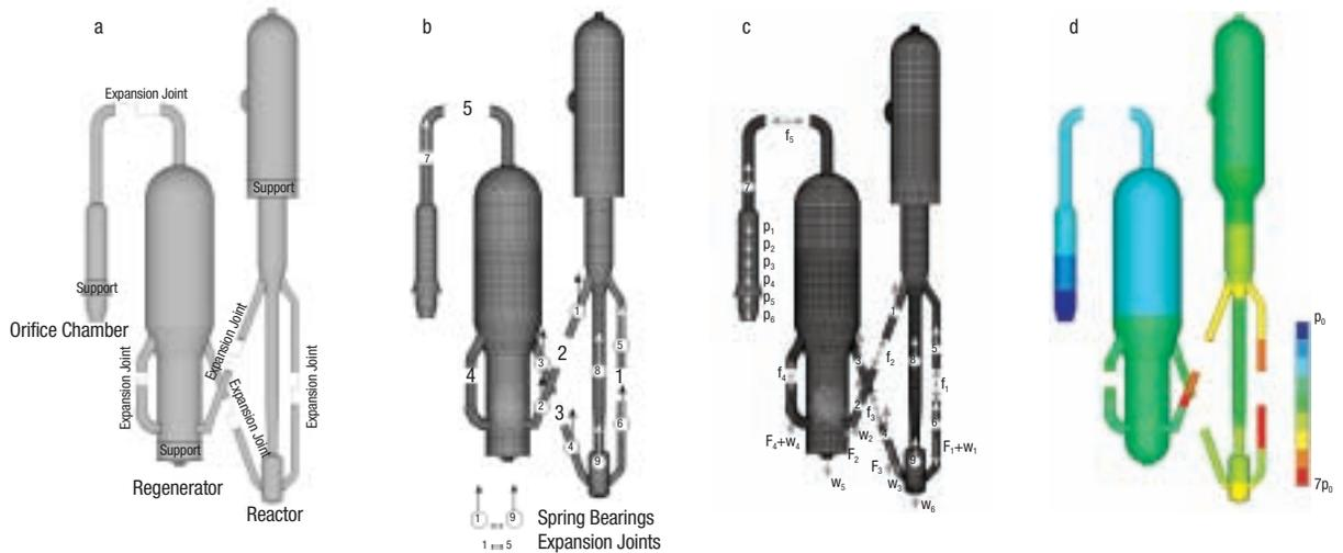
(a) 3-D solid model of the cracking system, (b) location of the spring bearings and bellows expansion joints, and vector (c) and contour (d) representations of the mechanical loads that are caused by internal and external pressures, gravity and catalyst density, and that are acting on the equipment
