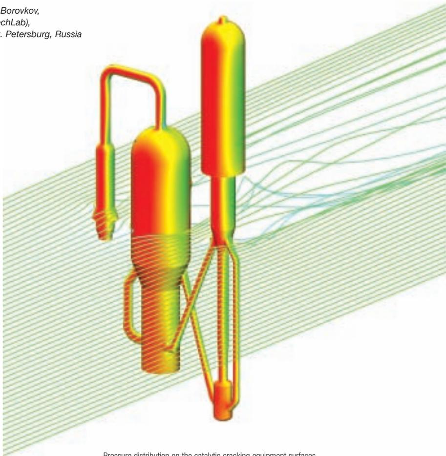
Pressure distribution on the catalytic cracking equipment surfaces due to the external air flow (represented by the streamlines)
