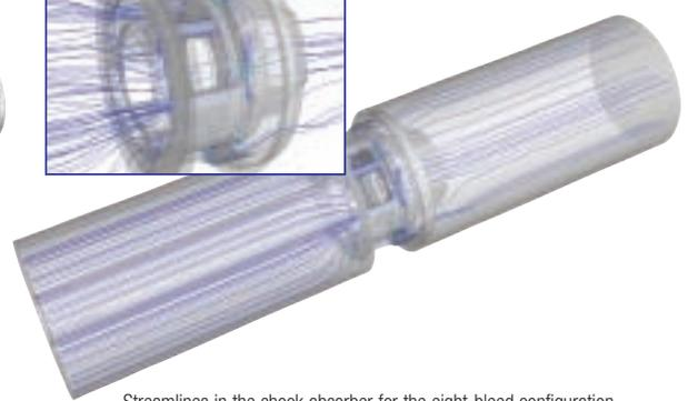
Streamlines in the shock absorber for the eight-bleed configuration
