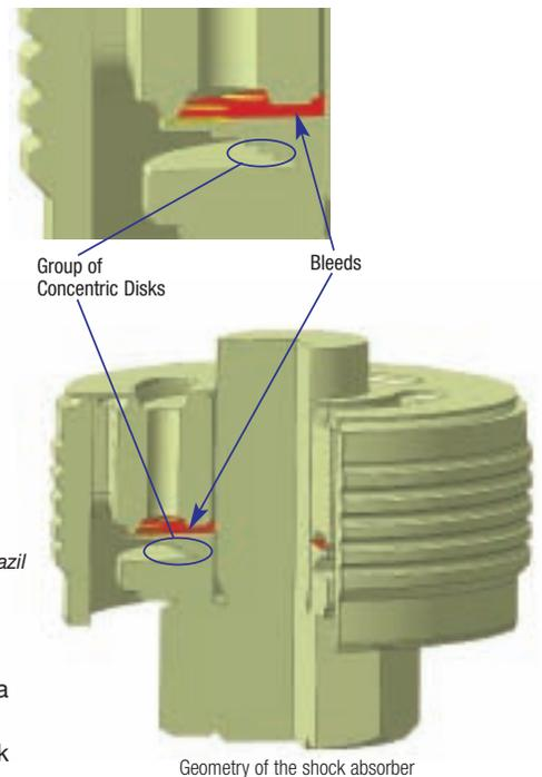
flow software. The team considered three configurations of bleeds (two, eight and 16 bleeds) under three velocity conditions for each configuration at the inlet. They obtained the pressure field on the regions of interest at the valve using the CFX-Post post-processor and generated a plot of force (at the valve) versus velocity. The results showed very good agreement with experimental data.
