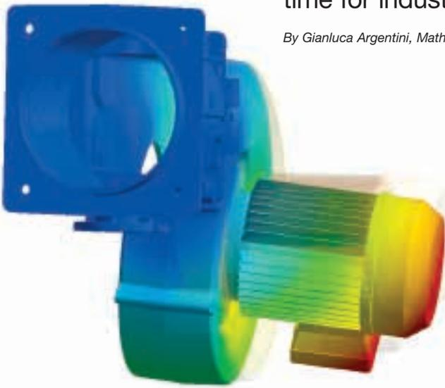
Displacement at the first natural vibrational mode for the original Riello burner configuration
