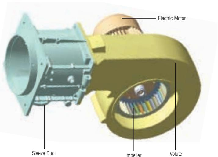
The geometry of a burner assembly: Air is taken in through the impeller and directed into the sleeve duct, which houses a combustion head (which initiates the flame).
