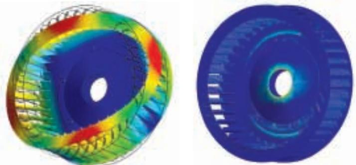
Impeller four-nodal diameter mode associated with its first natural frequency; this value, 141 hertz, is close to other vibrational frequencies of the global system.
