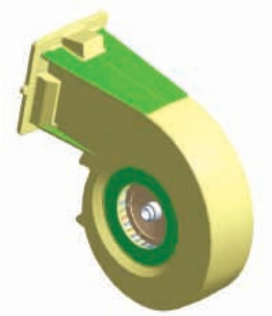
The new design of the volute showing reinforcement by ribs at upper and lower parallel surfaces and by new material at the engine flange (modifications in green)
