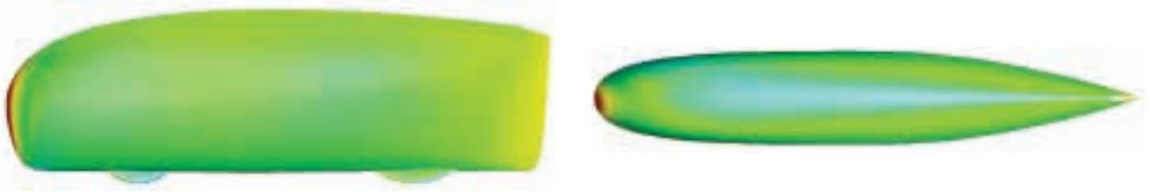
Pressure contour on exterior side (left) and top (right) of a speedbike, assuming a 4-degree diagonal flow
