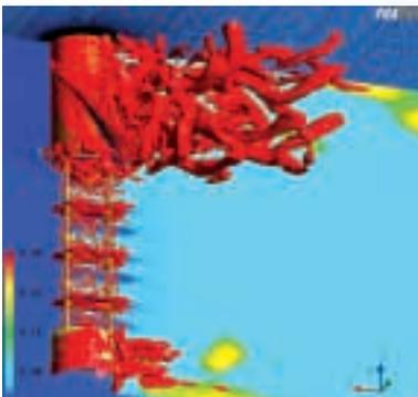
For environmental, green and sustainable design, engineers use simulation tools from ANSYS to evaluate retrofit options, optimize combustion and heat transfer, capture pollutants, design pipelines and sub sea equipment, look at safety and installation strategies, and increased structural integrity to avoid spills and disruption. Vortex-induced motion for this truss spar is modeled to understand global and local forces on the spar streaks. Geometry courtesy Technip U.S.A.
