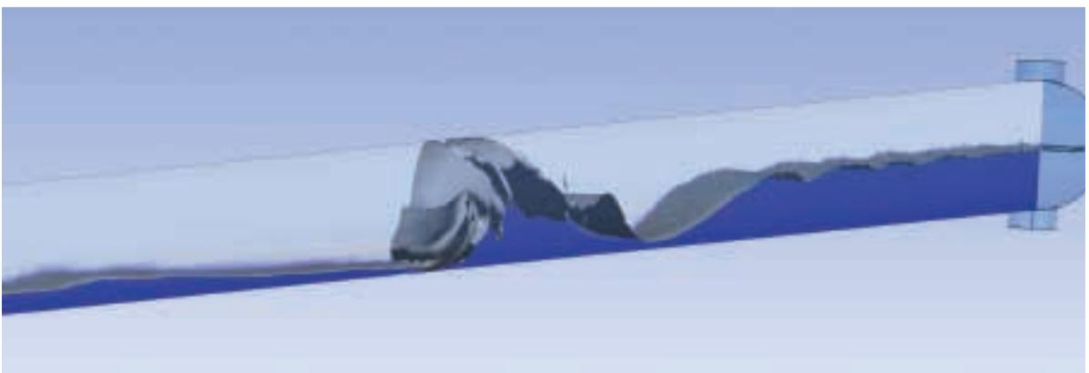
Technology from ANSYS is applied to flow assurance projects dealing with oil flow ability (addressing sand management, slug flow and gas-lift applications), ensuring more efficient and uninterrupted flow of oil in a given pipeline. This example shows slug flow in a gas-liquid pipeline.
