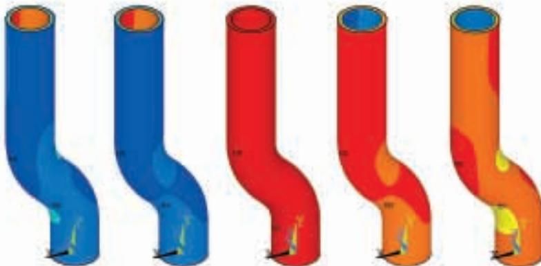
Temperature distribution in the pipe for typical heat-up and cool-down. From left to right: 10, 30, 70, 100, 130 seconds, with blue indicating lower temperatures and red higher temperatures
