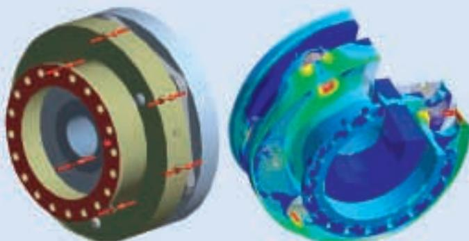
The assembly model includes pretension bolted joints and BISO material for the hub and spacer.
