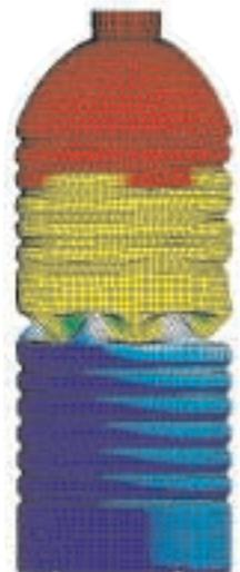
Top-loading simulation of a plastic bottle
