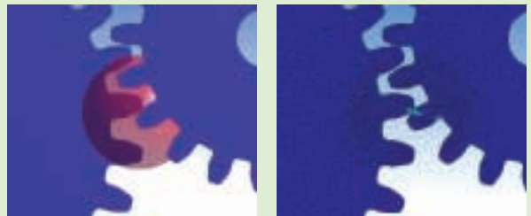
Figure 1. In an analysis of 2-D contact between gears, a SPHERE OF INFLUENCE (in red) is defined with a user-specified radius (left). This generates a fine mesh within this area for studying von Mises stresses at the point of tooth contact as well as within the geometry of the gear body (right).
