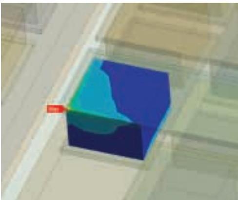
Structural analysis indicates the highest magnitude of stress on the corner of the thermoelectric element where Marlow has historically seen cracking.
