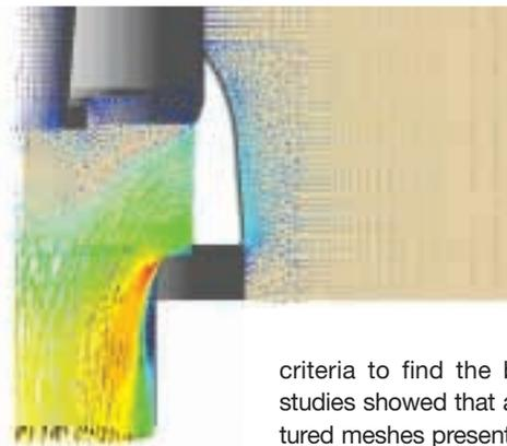
Water velocity vector field analysis inside the discharge valve
