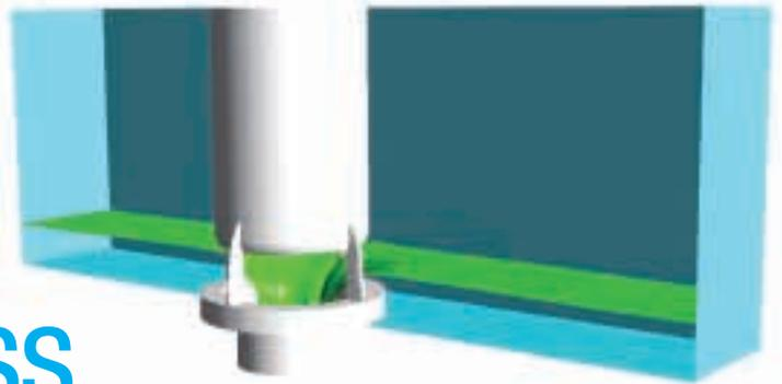
ANSYS CFX simulation results showing the free surface movement through the valve during discharge
