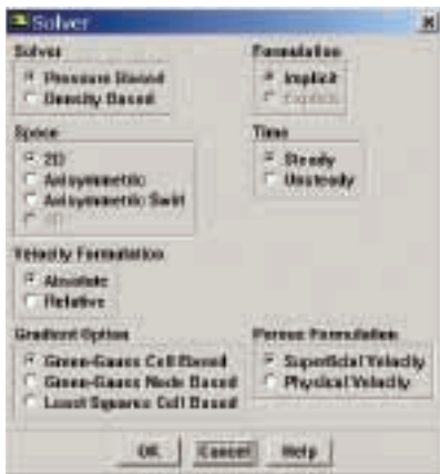
Figure 2. Selection of solver algorithms reflected in the Define→Models→Solver GUI (This panel was introduced as new in FLUENT 6.3.)
