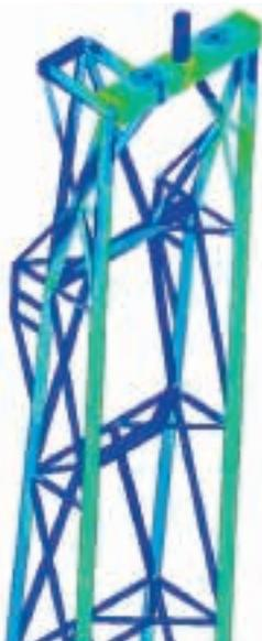
Von Mises stress simulation showing distributed stress along all elements of a derrick
