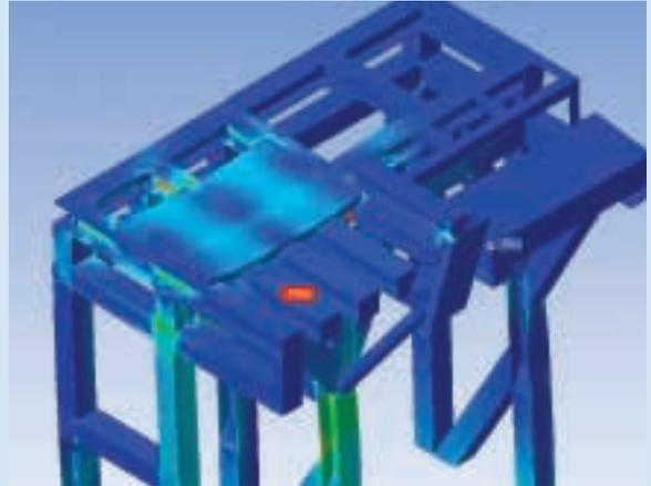
Von Mises stress contours on the substructure
