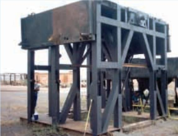
Derrick substructure at the yard for maintenance
