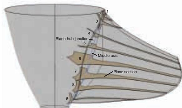
Definition of planes for fracture mechanics analysis. Intersection of the FMA with hubs and blades is shown.
