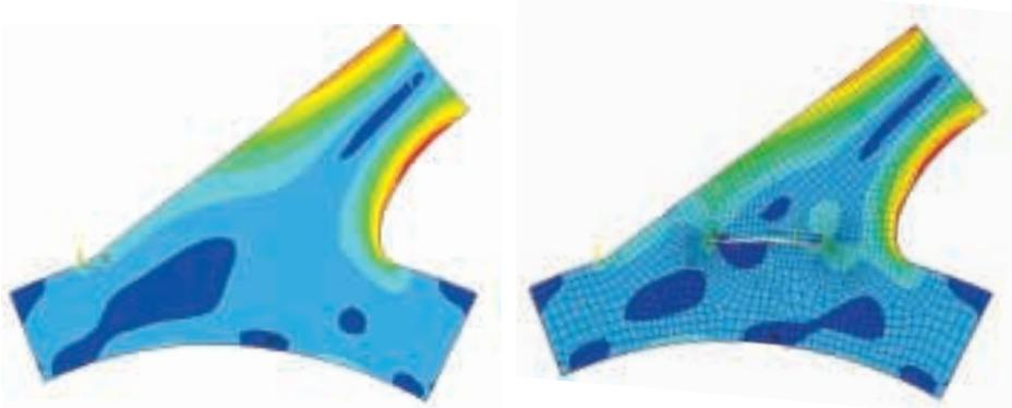
Comparison of stress intensity for the blade design used in the St. Lawrence runner with no defects (left) and with a partial penetration weld (right)
