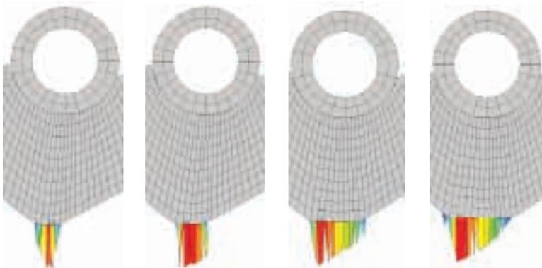
Evolution of seal wear from cycle to cycle: The change in the interface at the bottom of the seal area (lower grey edge) illustrates a change in shape; contact pressure is plotted across this lower edge, where the red areas indicate regions of maximum pressures of 19, 9.5, 3.4 and 1.6 MPa, from left to right respectively.
