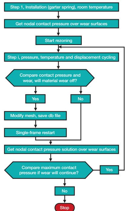
Simulation flow chart for single-frame restart procedure used for FEA modeling of a continuously wearing seal geometry
