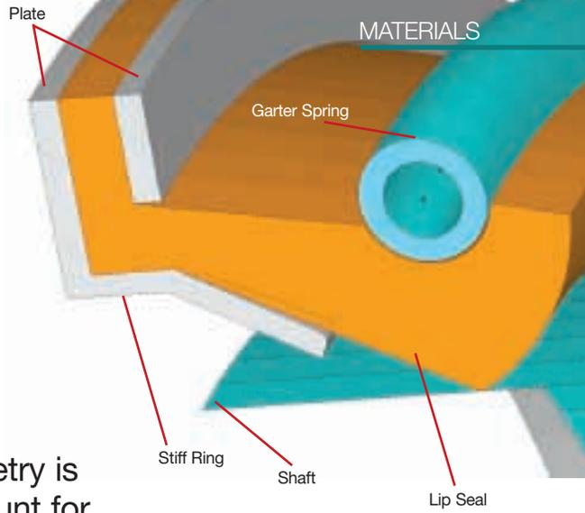
Radial lip seal geometry simulation model
