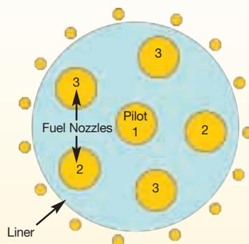
Diagram of a gas turbine combustor showing locations of burners that are operated depending upon required load. Numbers indicate burners that operate together for the various stages of operation.
