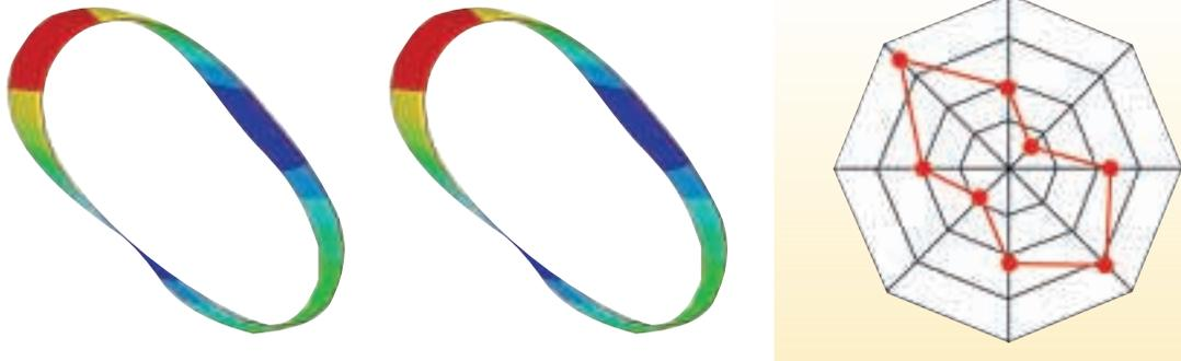
Simulation results for creep deformation at shutdown after 25 hours of part-load operation (left); 1,000 hours of part-load operation (center) and deformation as measured by CMM inspection after experimental testing (right). Deformed shape is exaggerated in FEA images.
