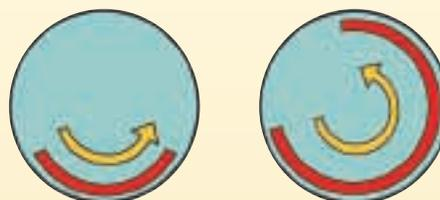
Red lines indicate the areas along the liner circumference that develop hot streaks when one stage (left) or two stages (right) are used.
