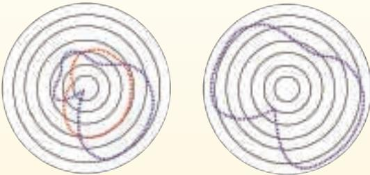
The difference between the overall hoop stress (blue, left diagram) and the hoop stress due to radial temperature (red, left diagram) yields the stress caused by the thermal asymmetry (right diagram). The values in the left diagram were calculated based on simulation results using technology from ANSYS.
