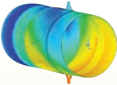
This contour plot of temperatures for the liner thermal plot (results for having two main stages on) shows a large circumferential metal temperature gradient on the liner surface over the entire length of the combustor. Orange indicates higher temperature, and blue indicates lower temperature.
