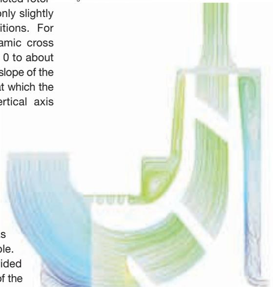
Figure 3. Streamlines through stage 1 at the instability point #1, 21,500 rpm
