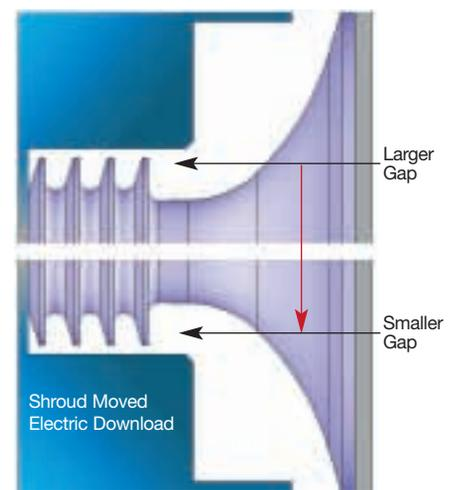
Figure 2. Geometry of compressor under study. Since only shroud forces are of interest in this study, only the shroud region is made eccentric.
