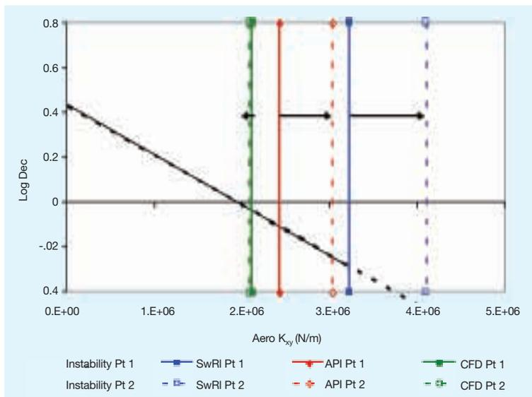
Figure 6. Stability curves for the compressor under analysis and various predicted values for which the compressor would become unstable (i.e., prediction values for where the curves would cross the x-axis of this plot; the CFD results provide the most accurate prediction).
