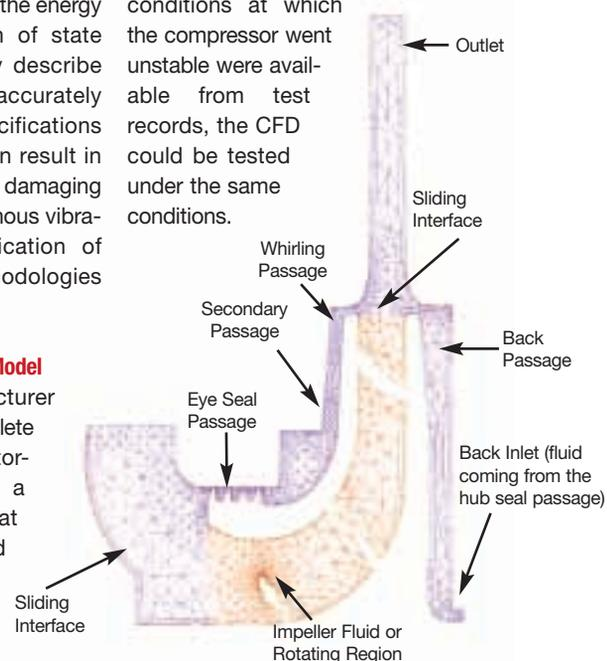
Figure 1. The compressor mesh with the boundary condition surfaces and sliding interfaces
