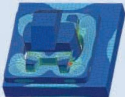
Stress analysis of a container lock mechanism
