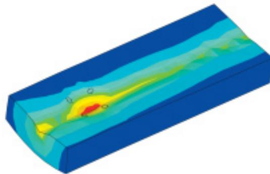
Numerical results for membrane deformation ( $\mu\text{m}$  units)
