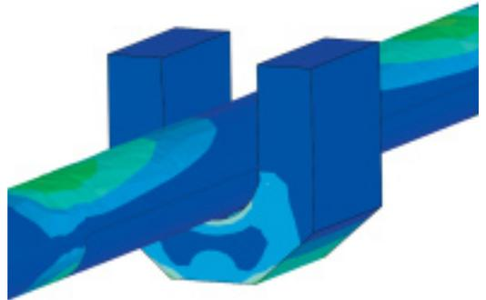
FEA was used to determine contact forces on sensor strips in the surgical device.
