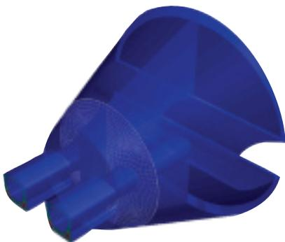
Fluid model extracted from solid CAD model
